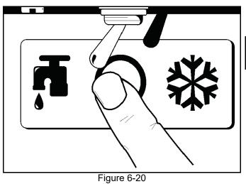
5. Place an empty pail beneath the door spout and move the draw handle to the right. Draw off all the sanitizing solution. When the sanitizer stops flowing from the door spout, move the draw handle to the left and place the control switch in the OFF position.
