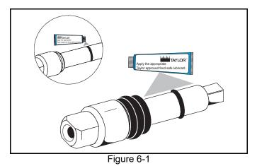
Note: Do not install the boot seal inside out.
