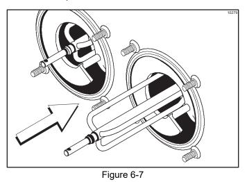
Before assembling the freezer door, check the following for any nicks, cracks, or signs of wear: front bearing, door gasket, draw valve, O-rings, and all sides of the door assembly, including the inside of the draw valve bore. Replace any damaged parts.
